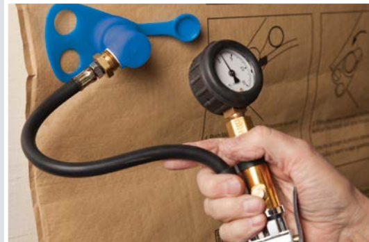
Use pressure gauge when filling. Use tool model 2910-6983-HD-KIT.
