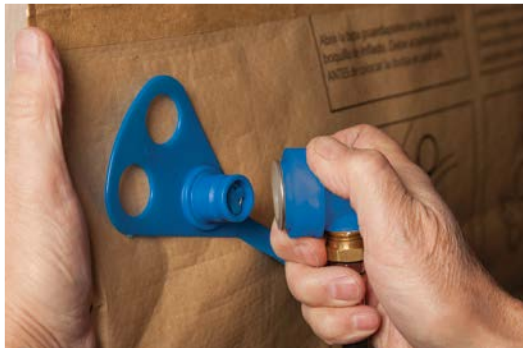
Attach quick-connect lock-ring tip to filler valve.
