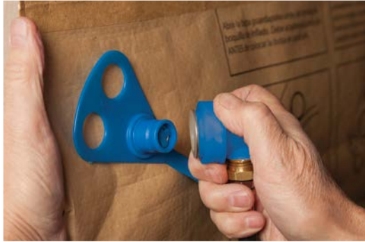
Attach quick-connect lock-ring tip to filler valve.
