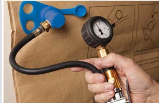
Use pressure gauge when filling. Use tool model 2910-6983-HD-KIT.
