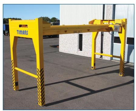
This overheight frame has been developed to meet the increased safety demands in ports, and is equipped with a new electrical system with IFM PLC, alloy steel actuators, several smart safety features and a very smart, power-saving sleep mode. The OHE can also be equipped with the new Hoist Interlock system and service communication system.
