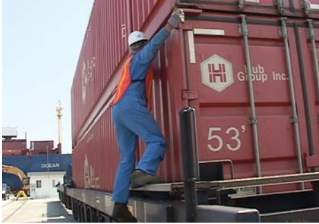
Prevent fall by locking & unlocking from the ground with a pole.
